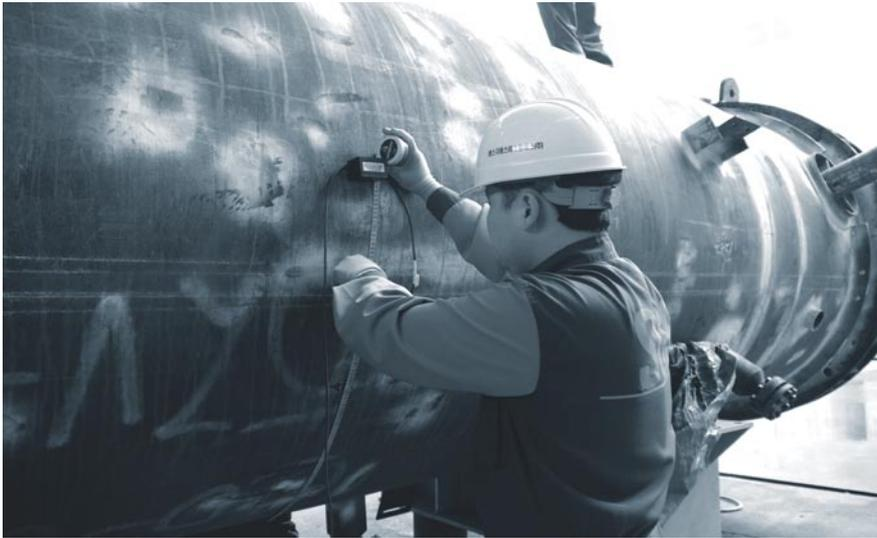
Acoustic Emission Testing (AET) is a Non-Destructive Testing (NDT) method that is used to analyse emitted sound waves caused by defects or discontinuities. These acoustic waves are induced by small deformations, corrosion or cracking, which occur prior to structure failure. It is therefore possible, with AET, to locate structural defects and to monitor the propagation and development of discontinuities.
